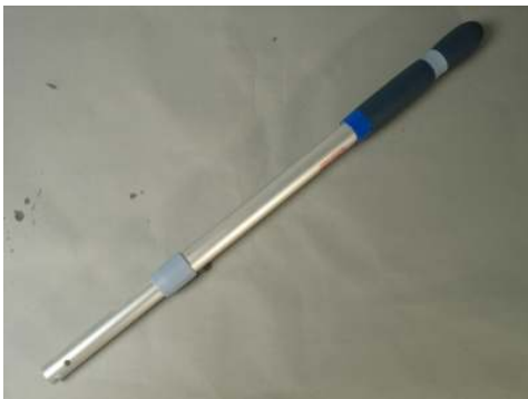
Photo 1: Telescopic Handle frame after 80 cycles
