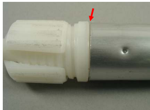
Photo 2: Inner screw becomes a bit loosen
