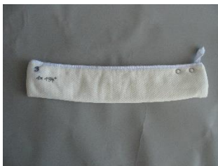
Photo 1: MicroIntensive™ L Cover after 1 autoclaving cycle
